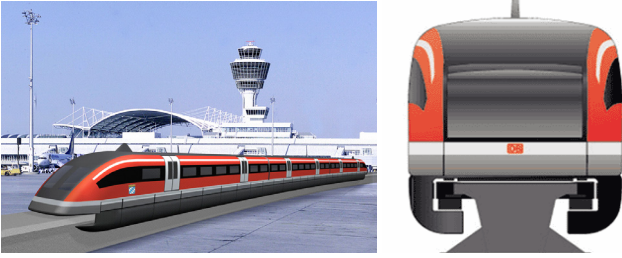
Figure 2: Artist impression of the maglev link at the airport and the layout of the guideway (Illustration of BMG)
