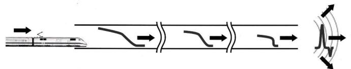
Figure 1: Illustration of development of micro-pressure waves.
