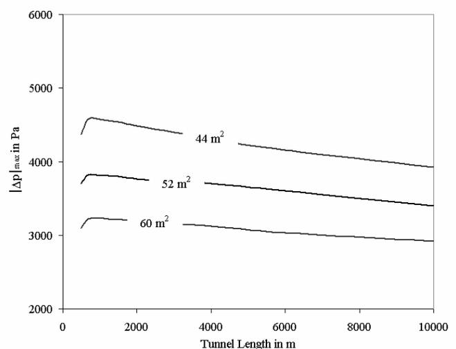
Figure 2: Maximum pressure variation  $|\Delta p|_{\max}$  acting on a 12.4 m<sup>2</sup>-train in a tunnel with respect to tunnel length and tunnel cross-section (single-track tunnel, no pressure waves of other trains, no shafts, train length 100m, train speed 250 km/h).
