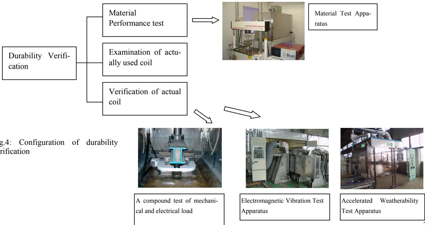
Fig.4: Configuration of durability verification
