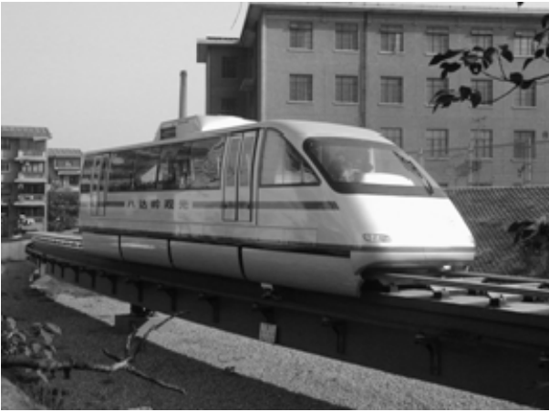
Figure3: the CMS-03 type magnetic suspension train developed in 2001 is running on the experimental line
