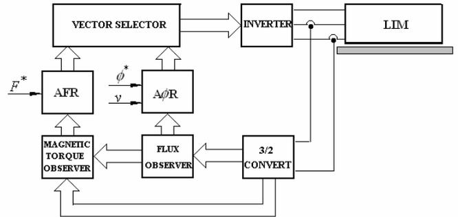
Figure 7: The ordinary control method
