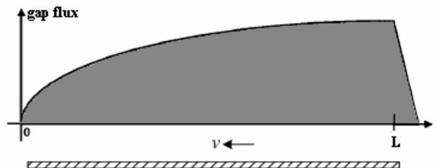
Figure 1: Gap flux distribution along the primary
