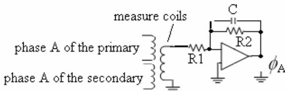
Figure 5: Integration circuits for flux
