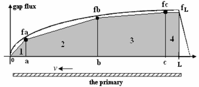
Figure 6: Gap flux approximation
