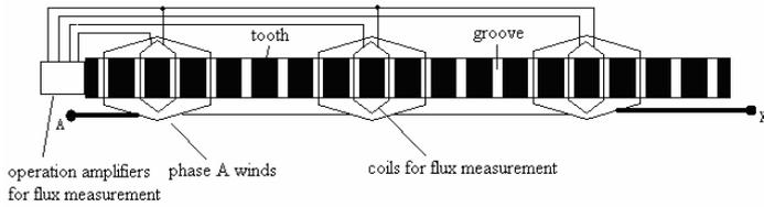
Figure 3: Lines connect coils to circuits
