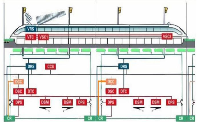
Figure 2: Components of the operation control system
