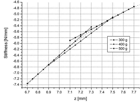
Fig. 9: Stiffness vs. displacement and the weight of the levitation-part
