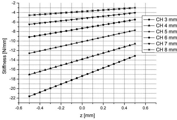
Fig. 7: Vertical stiffness vs. vertical displacement
