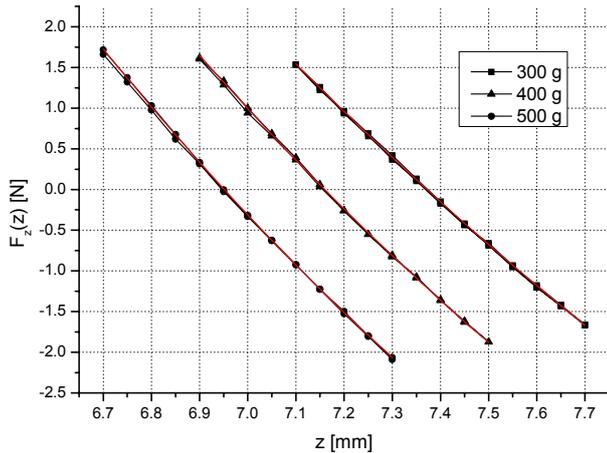
Fig. 8: Curve fitting to calculate the stiffness at three work points due to the weight of the levitation-part
