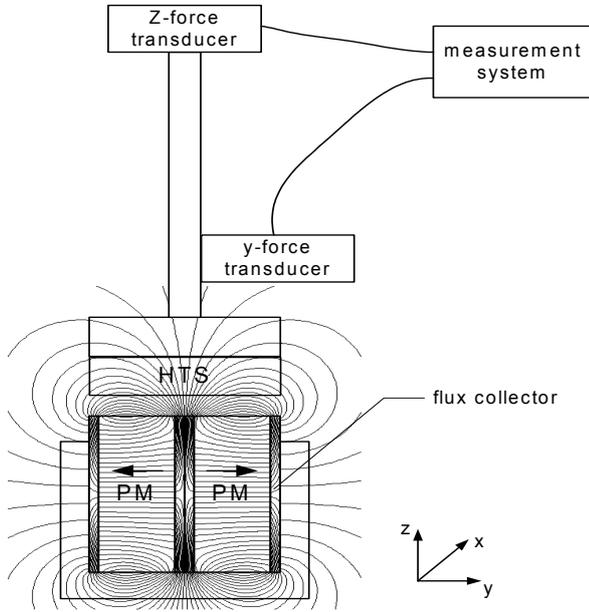
Fig. 1: System for measuring static force and stiffness
