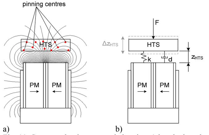
Fig. 11: Superconducting magnetic bearing a) is substitute by a mechanical oscillation model b)
