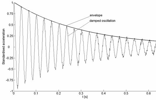
Fig. 10: Damped mechanical oscillation and envelope of the levitation-part
