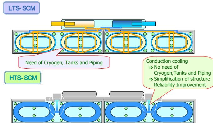
Figure 4: The structural comparison between LTS and HTS
