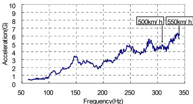
Figure 3: The acceleration of the new-type SCM
