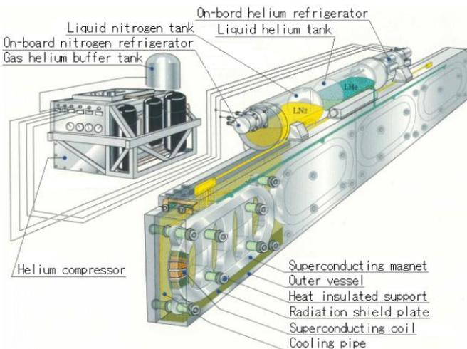
Figure 1: The schematic view of the SCM
