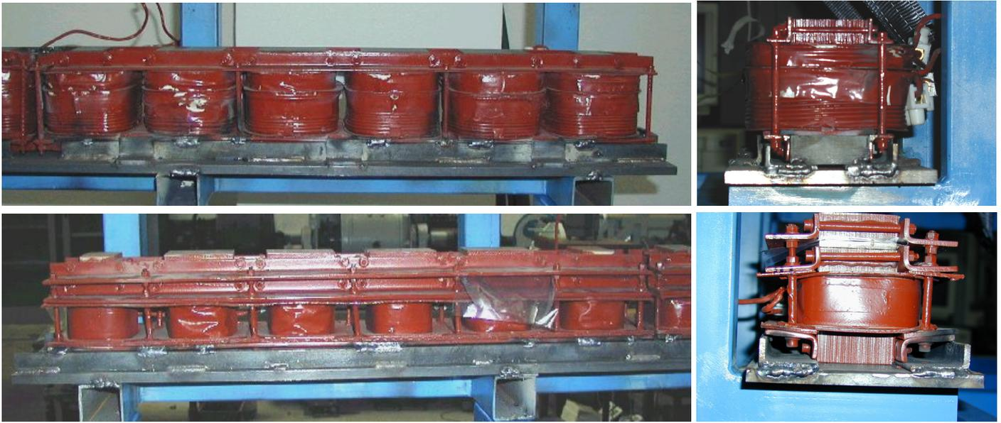
Figure 3: photos of the esapolar levitation units. Upper: CO type. Lower: PMs type.
