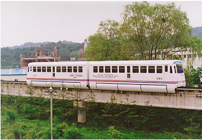
Figure 5: Photograph of experimental vehicle for magnetically levitated transport system
