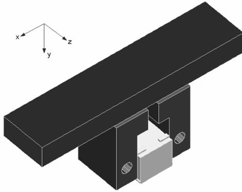
Figure 3. 3-D drawing of the levitation axis – single coil.
