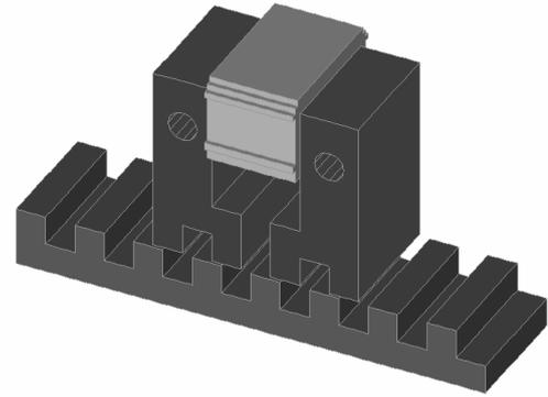
Figure 5. 3-D drawing of the propulsion axis – single phase.
