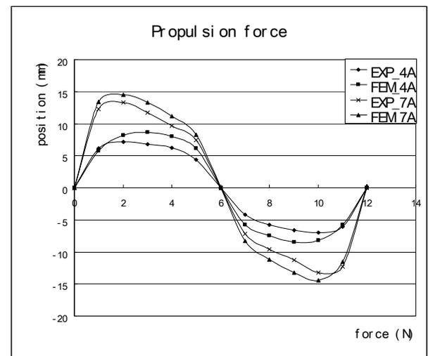
Figure 7. Propulsion force of the propulsion actuator.
