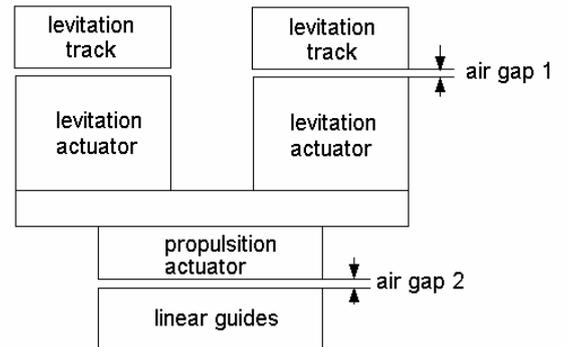
Figure 2. Side view of the proposed actuator.
