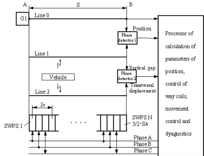
Figure 5: The LSD Maglev control system counter.
