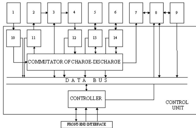
Figure 4: The SWPS block diagram: 1 – solar panel; 2 – electrolytic tank; 3 – hydrogen storage; 4 – fuel element; 5, 6 – accumulative batteries; 7 – ionistor; 8 – inverter; 9 – guide-coil; 10 – input electrical energy counter; 11 – charge counter; 12 – consumption counter; 13, 14 – charge-discharge counter
