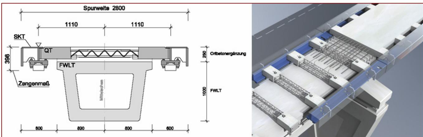
Figure 2: Track of Type II, BGmU design (Source: BGmU)
