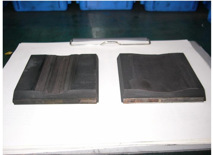
Figure 7: Comparison of power collecting pad
