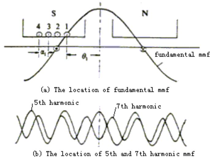
**Fig.2 The location of conductors 1,2,3,4 in the field of 5<sup>th</sup> and 7<sup>th</sup> space harmonics when  $\psi_0=0$**
