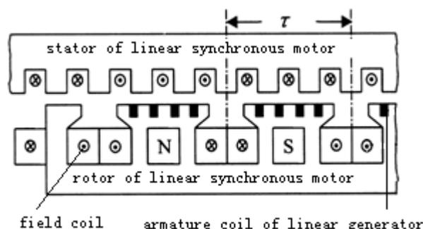
**Fig.1 The principle of linear generator**
