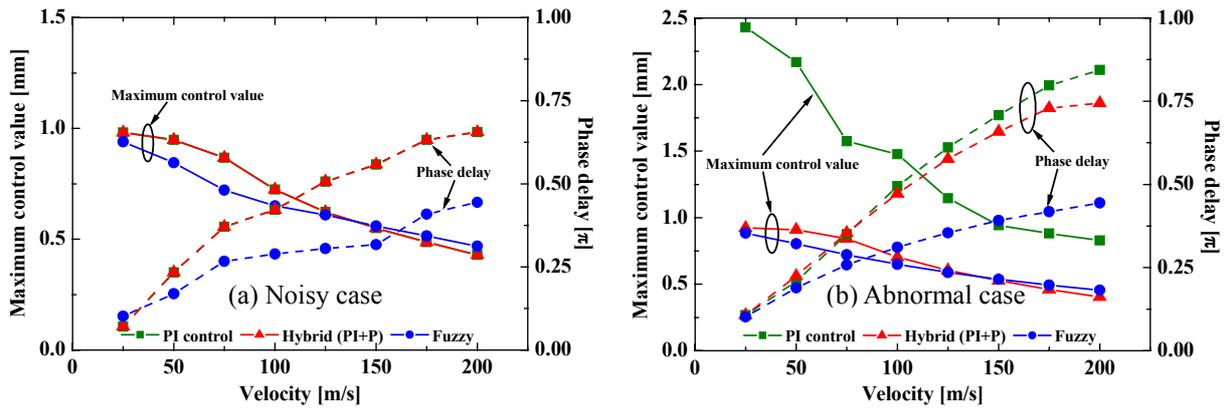
Fig. 17. Comparison of control performances based on maximum control value and phase delay for each
