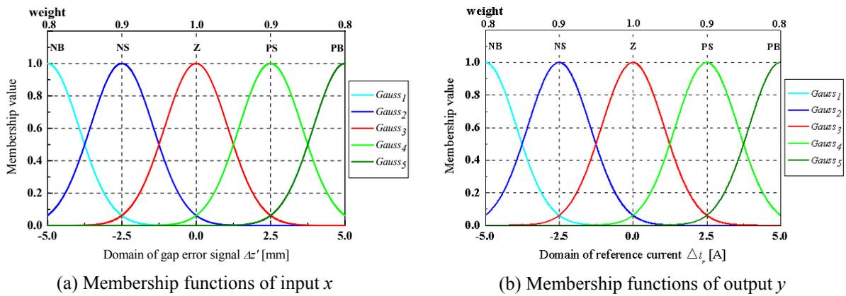
Fig. 8. Membership functions of fuzzy label ([B: big, S: small, N: negative, Z: zero, P: positive])
