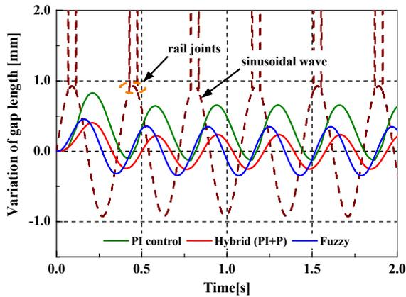
Fig. 14. Variation of gap length against an abnormal input at rail joint
