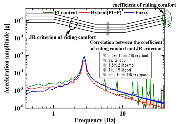
Fig. 16. Frequency characteristics of vertical acceleration of the cabin
