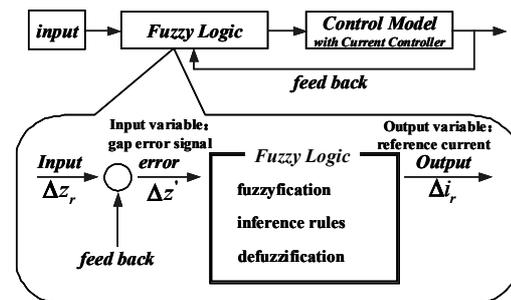
Fig. 7. Concept of gap length control with fuzzy logic
