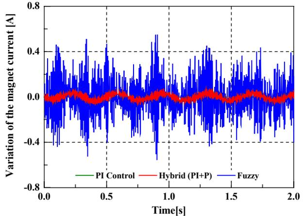
Fig. 10. Variation of the magnet current
