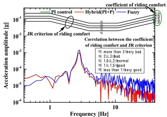
Fig. 11. Frequency characteristics of vertical acceleration of the cabin
