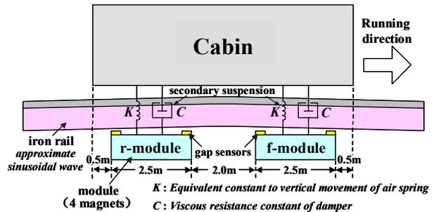
Fig. 3. Magnetic levitation model
