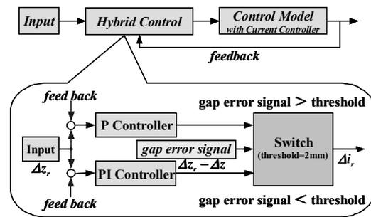
Fig. 6. Concept of hybrid control scheme
