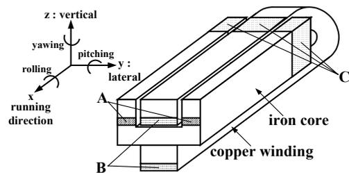
Fig. 18. Image of smaller magnet
