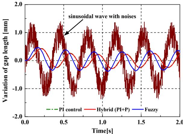
Fig. 9. Variation of gap length against the rail alteration with noises
