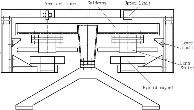
**Fig. 1. The cross section of the proposed hybrid levitation system**
