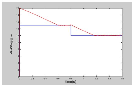
(d) step response from 15mm to 12mm for expert PID control
