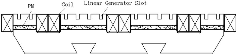
**Fig2. The structure of the hybrid magnet**
