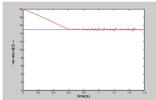
(c) sudden load enhancement by 40% at 0.8s for expert PID control
