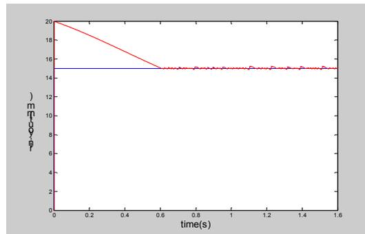
(b) normal levitation for expert PID control
