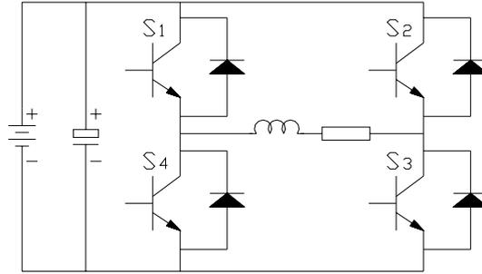
**Fig.3. The topology of the DC chopper**
