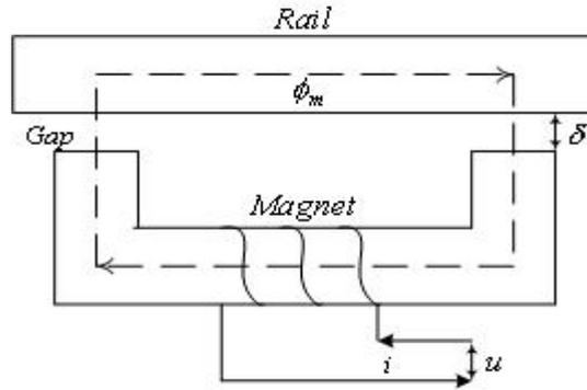
Fig.3 The magnet shape and magnetic field
