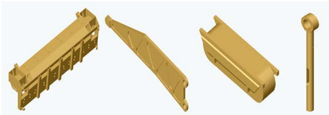
Fig.1 The main components of maglev bogie
