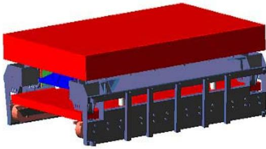
Fig.2 The maglev bogie model
