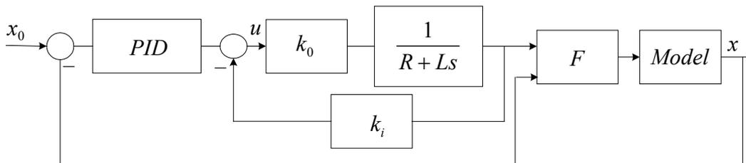
Fig.4 System transfer function diagram
