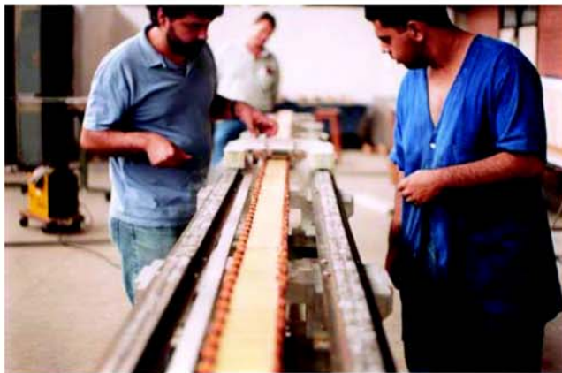
Fig. 7. (a) NdFeB levitation rails and linear motor rail.
