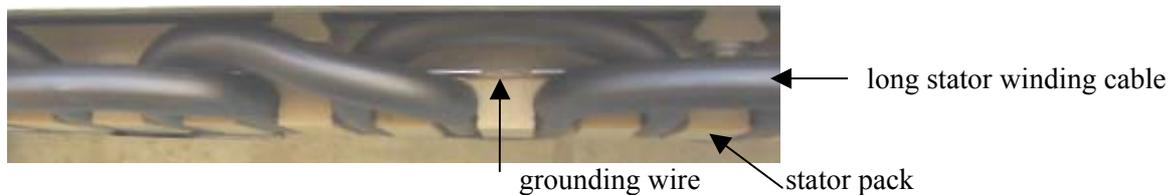
**Fig. 1: Present design of the motor winding of the Transrapid**
