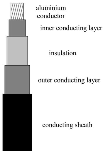
**Fig. 2: Long stator winding cable**
