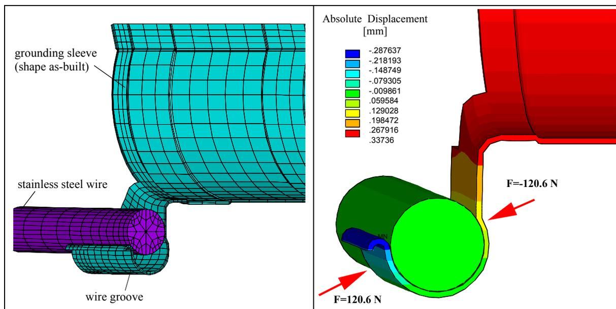
**Fig. 4: Model for calculation of the contact force using FEM (left side) and example for result of calculation (right side)**
