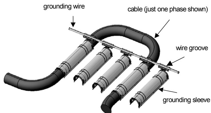
**Fig. 3: Grounding system of the motor winding (without stator packs, just one phase is displayed)**
