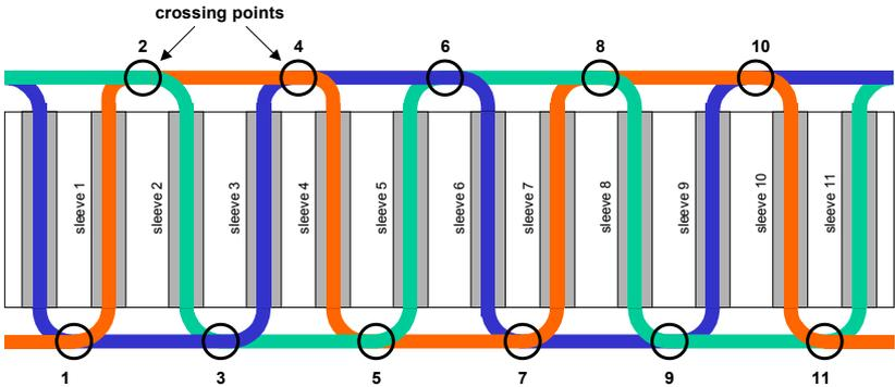
**Fig. 6: The principle structure of the three phases of the motor winding by highlighting the contact points (crossing points) between the end windings of the different phases**
