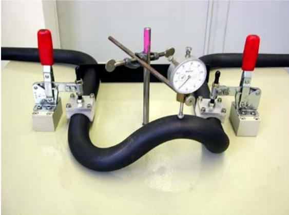
**Picture 8 : Plan-table for test of the form stability**
