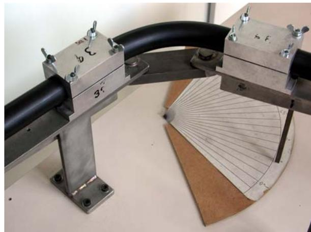
**Picture 6 : Test of manual bending property**
