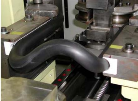
**Picture 7 : Bending/crimping unit (phase 2)**
