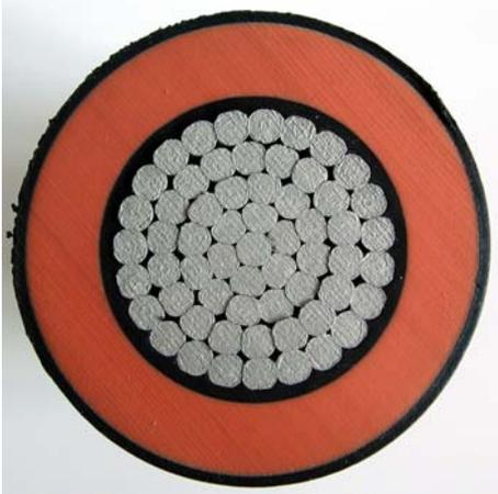
**Picture 4 : Standard conductor**
