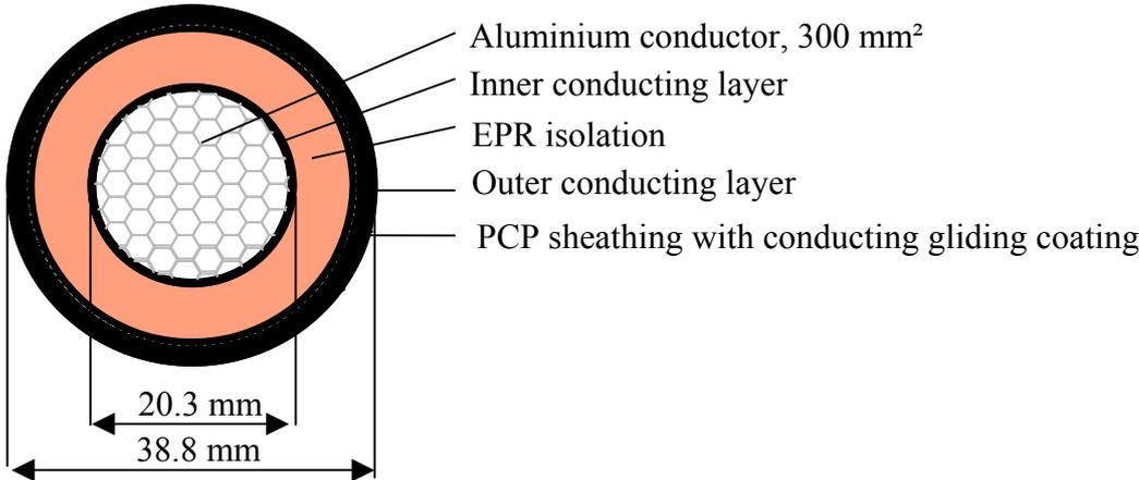
Picture 2 : Design of the LSW cable
