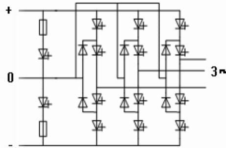
**Fig.2 The structure of the inverter module**
