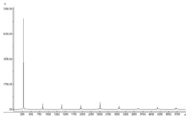
**Fig.7 The spectrum of the FFT of the output voltage**
