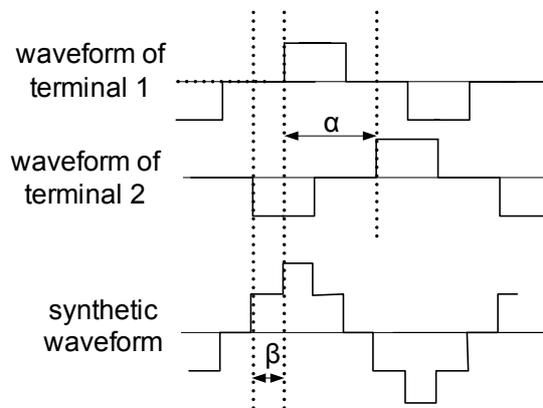
**Fig.5 The waveforms of the primary winding of the output transformer**
