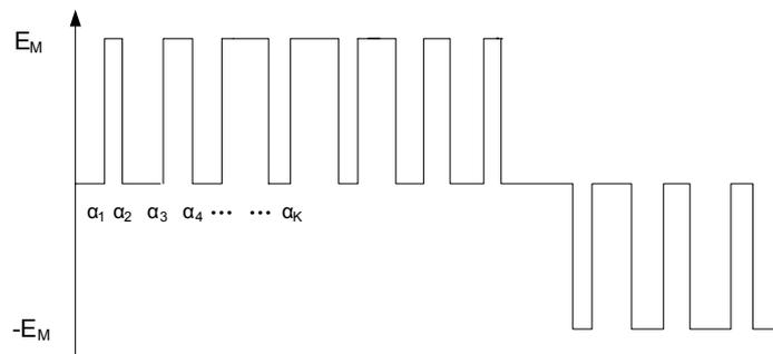
**Fig. 3 The three-level PWM waveform**
