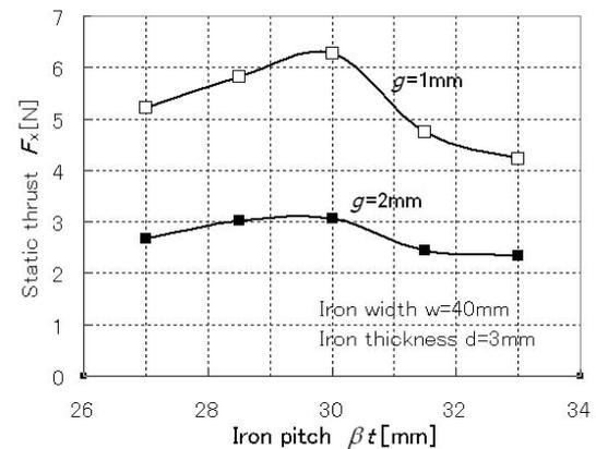
**Fig. 6 Maximum thrust depending on iron pitch.**
