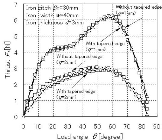
**Fig. 10** Load angle characteristics with or without tapered edge.
