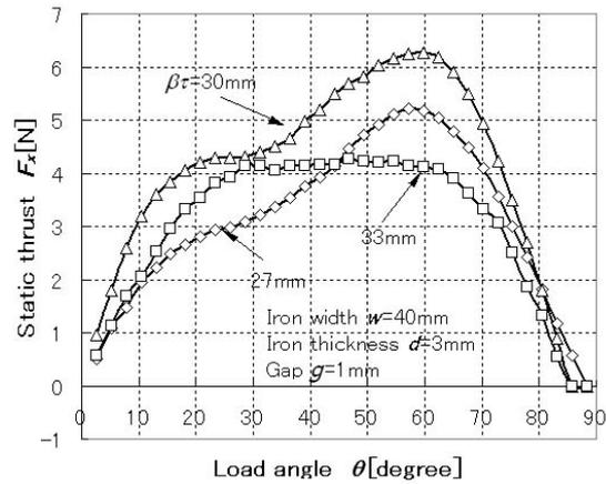
**Fig. 5 Static thrust vs load angle characteristics for different iron pitch.**
