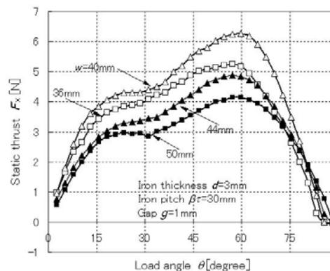
Fig. 3 Static thrust vs load angle characteristics at different secondary iron width.
