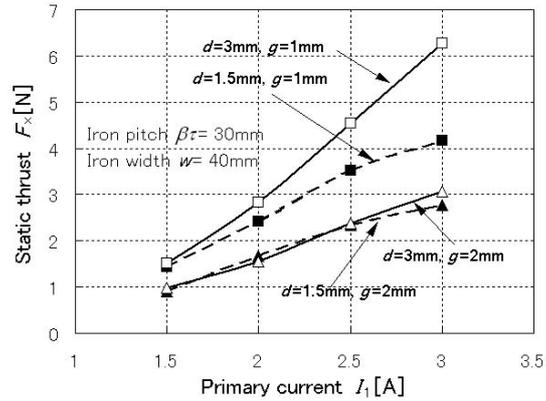
**Fig. 9** Maximum thrust depending on primary current.
