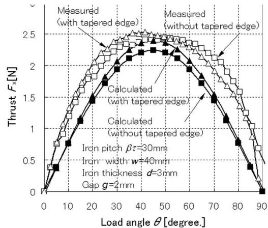
Fig. 13 Load angle characteristics in 4-pole double-sided test machine.
