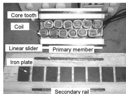
Fig. 1 4-pole single-sided test machine.
