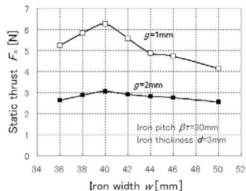
Fig. 4 Maximum thrust depending on iron width.
