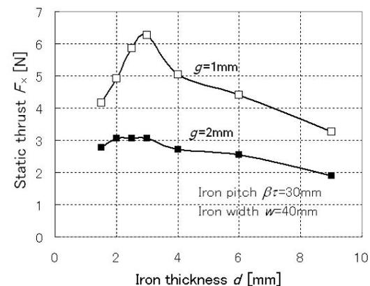
**Fig. 7 Maximum thrust depending on iron thickness.**
