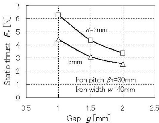
**Fig. 8** Maximum thrust depending on airgap length.
