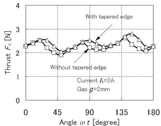
**Fig. 14 Instantaneous waveforms of thrust at load angle 45 degrees.**
