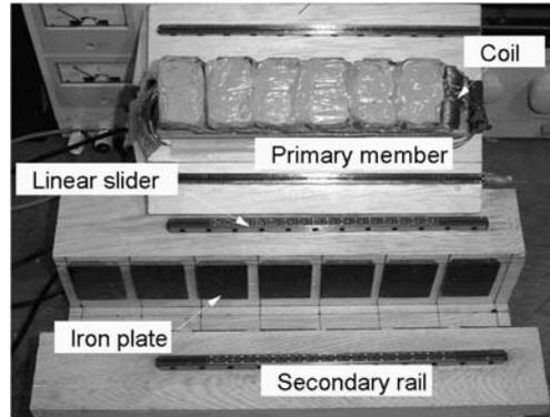
Fig. 2 4-pole double-sided test machine.
