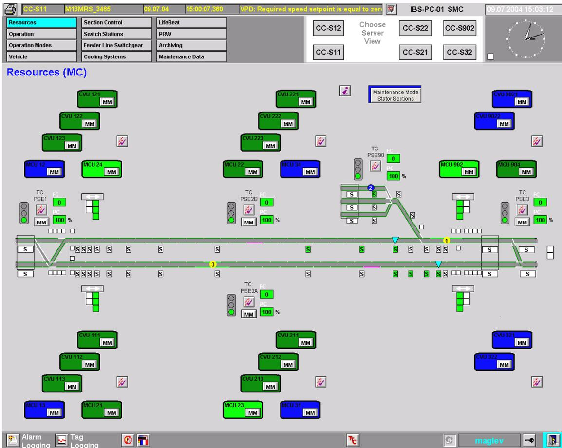
Figure 5: Propulsion layout of the Shanghai project as displayed in the operating and monitoring system
