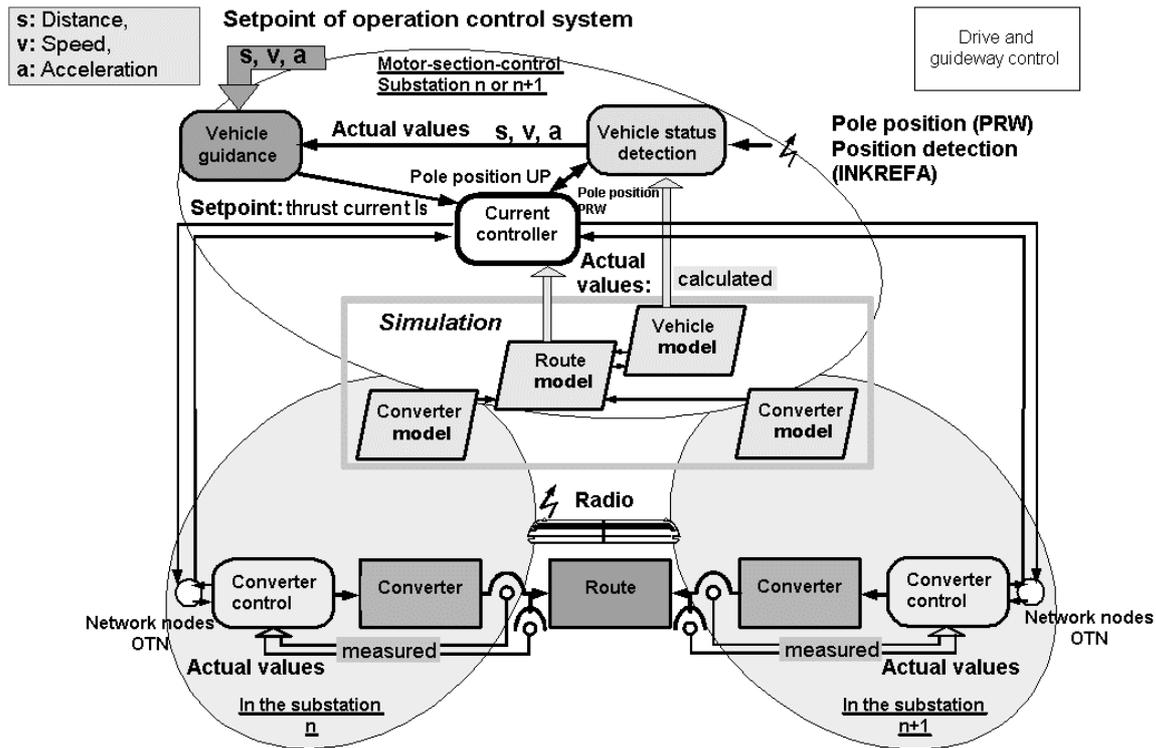
Figure 3: Basic functional units of the control system
