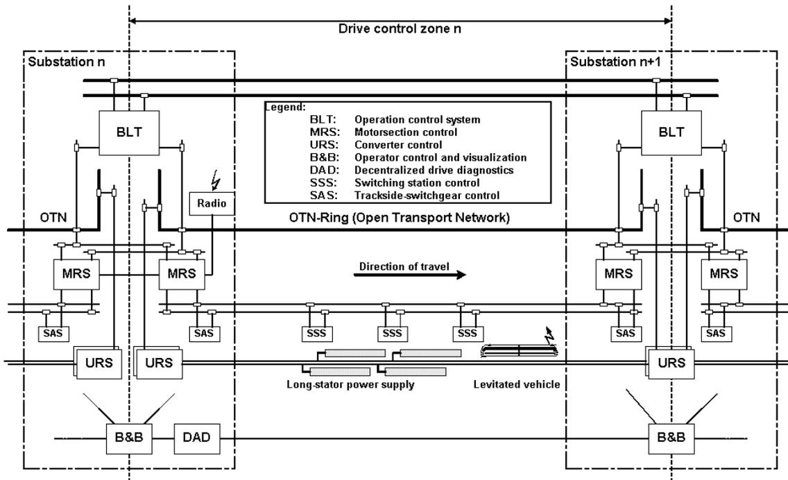
**Figure 2: Architecture of the drive control system**
