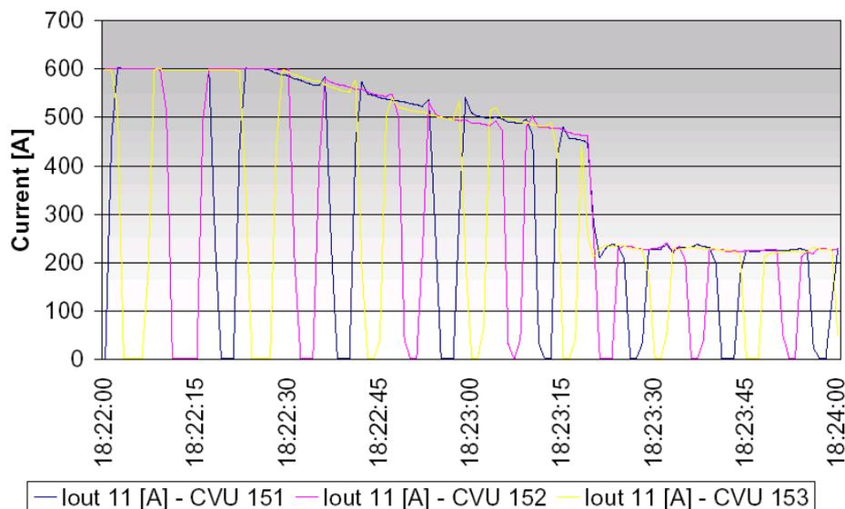
**Figure 8: Output-currents of the converters - three step method**
