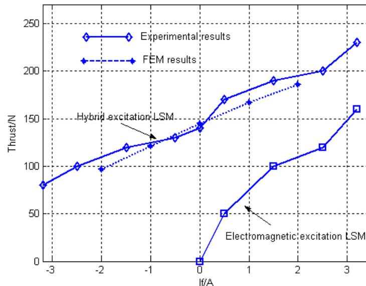
**Fig.4 Thrust-electrical excitation current characteristic curves**
