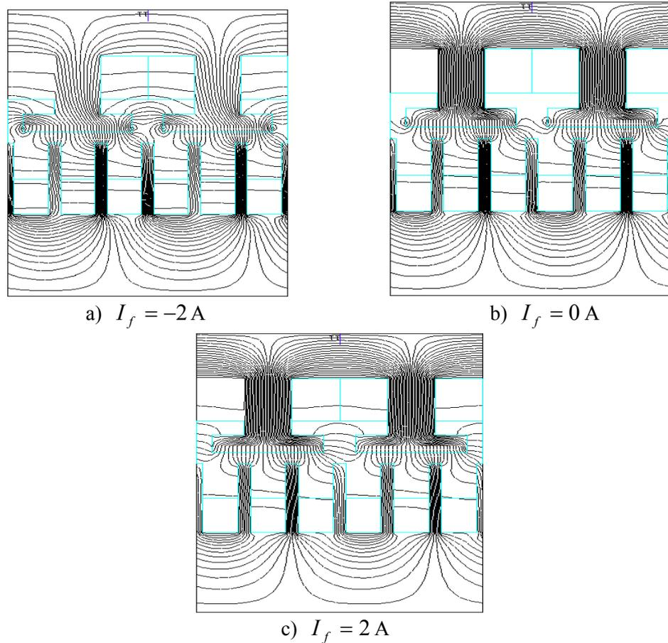
**Fig.2 The airgap magnetic field of one pole pair**
