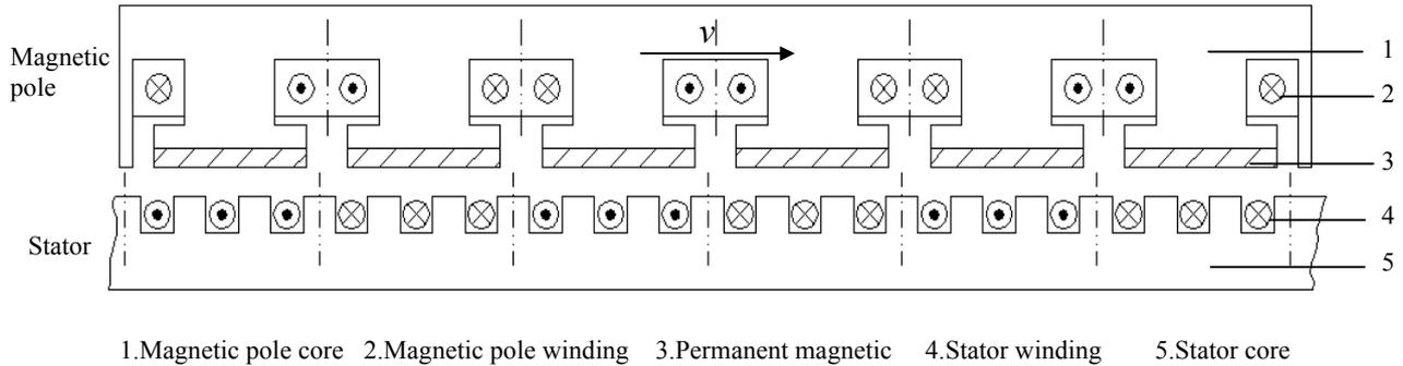
**Fig.1 Structure of hybrid LSM with permanent magnet and electrical excitation**
