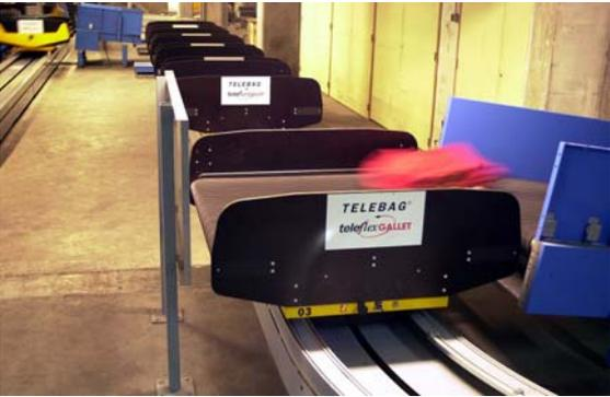
Fig. 2: TELEBAG cart loading a bag from a belt conveyor
