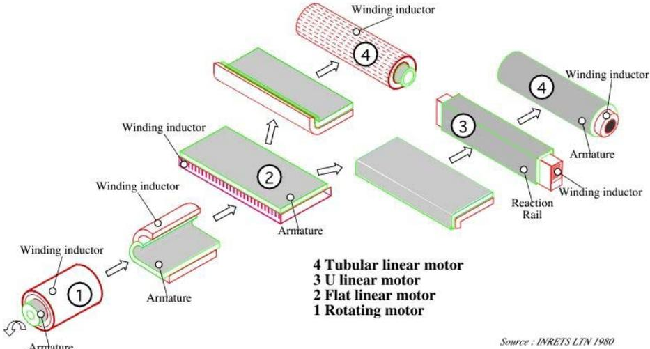
**Fig. 4: Ways for different LIM structures**
