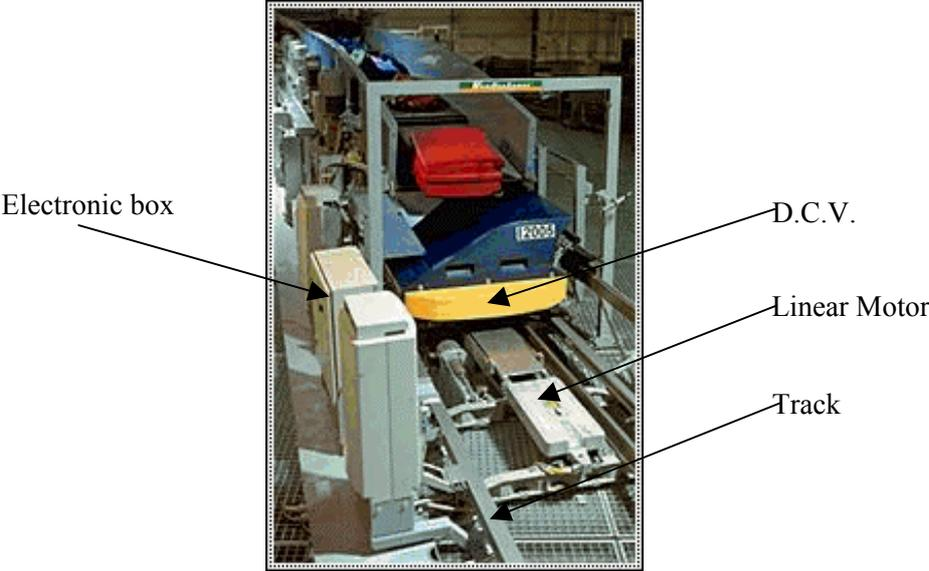
Fig. 1: Photograph of a D.C.V. at loading station
