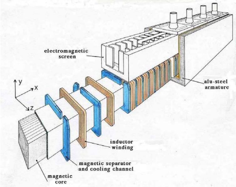
**Fig. 5: U shape reaction rail LIM (Celduc source)**
