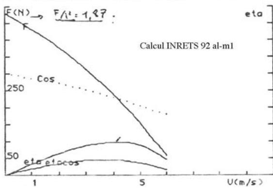
**Fig. 7: Mechanical thrust, power factor and efficiency**
