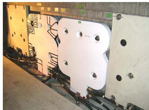
Fig. 8 PLG coils at the Yamanashi maglev test line
