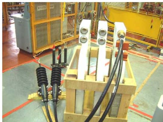
Fig. 7 Impulse dielectric breakdown test
