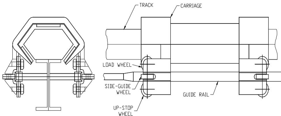
**Figure 2, Guide Wheel Arrangement**
