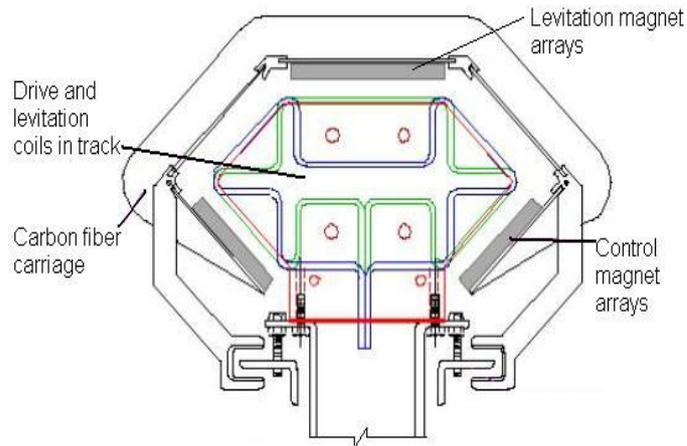
**Figure 1, Current Inductrack Configuration**
