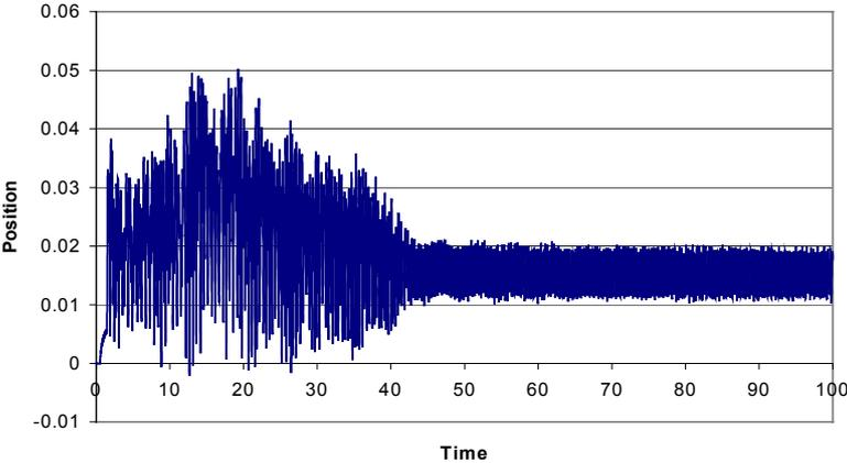
**Fig. 5. Vertical Position with Pitch Perturbation**
