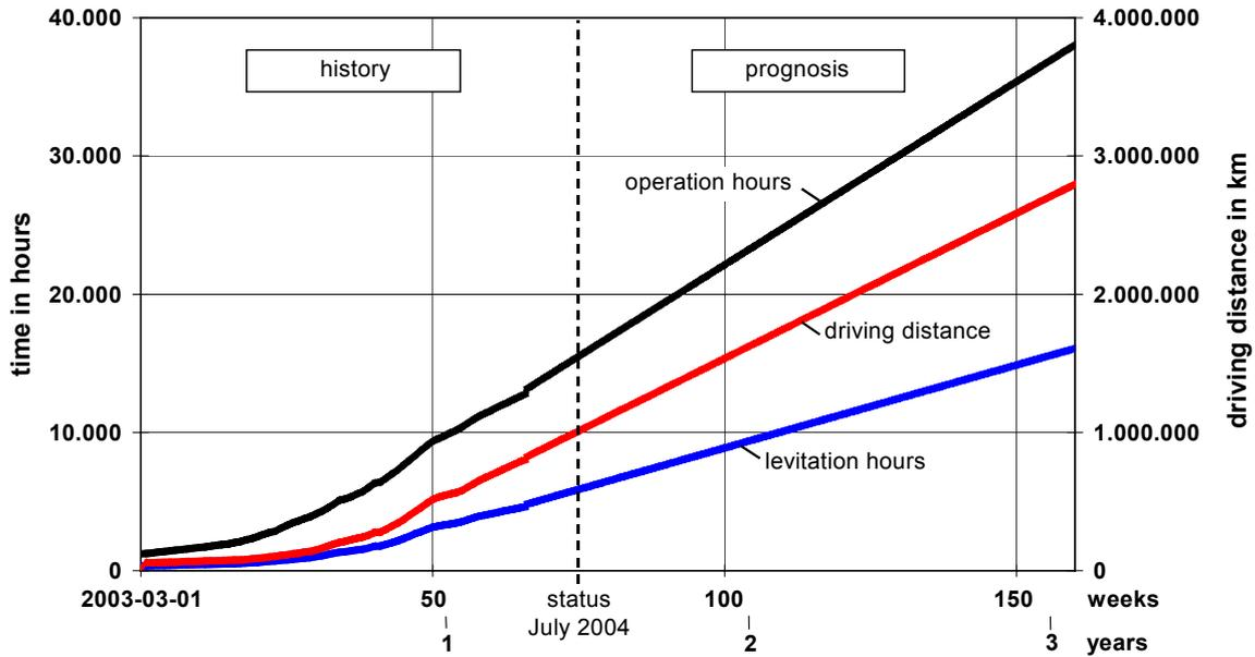
**Figure 2: operation data of Shanghai Transrapid vehicles**
