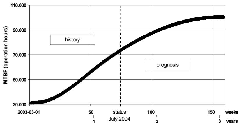
**Figure 3: MTBF of electrical components of the vehicles**
