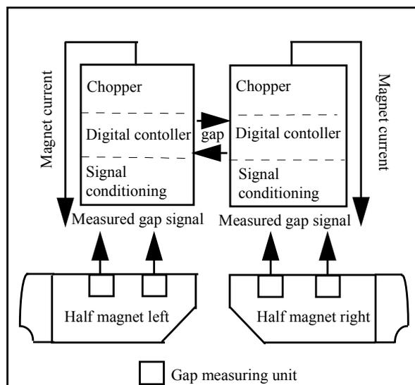
**Figure 1: Levitation frame with two control circuits**
