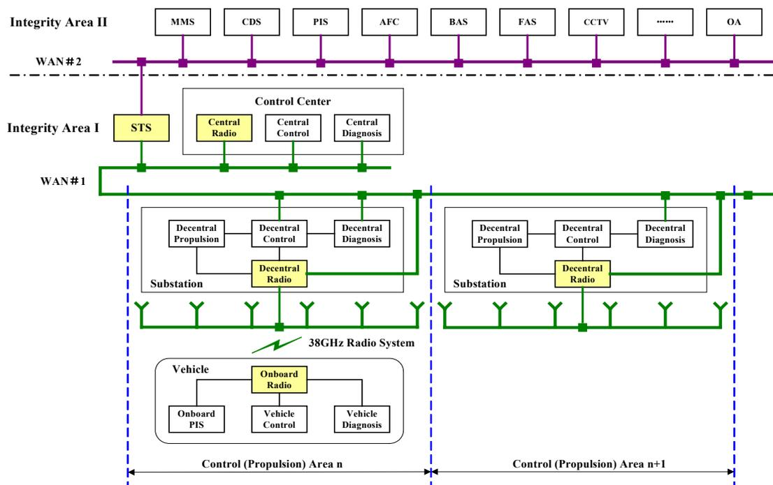
Figure 1 Sketch map of the backbone transmission network
