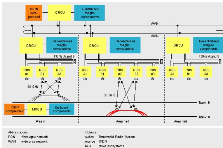
Figure 1 Structure of the Radio System
