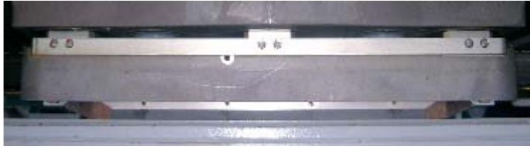
Fig. 2 Support skid with gliding elements.
