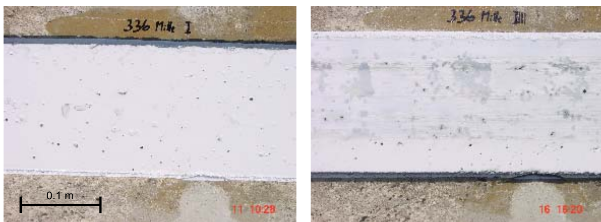
Fig. 6 Gliding strip after the first (left) and the 22 nd crossing of the support skid.
