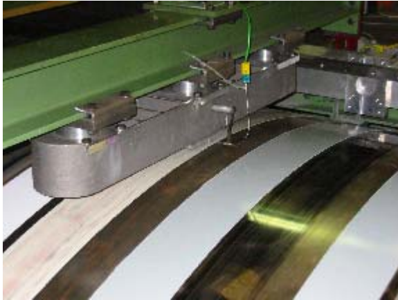
Fig. 4 Roller drum test rig with support skid.
