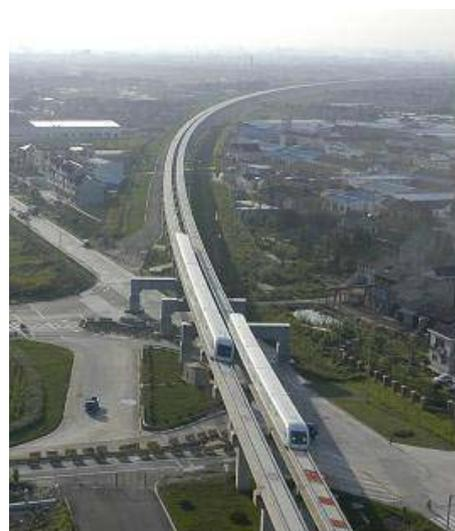
Figure 12: Shanghai Maglev Transrapid Vehicle Pass-by
