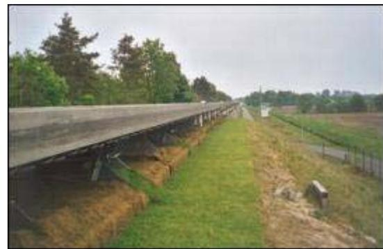
**Figure 7: Plate guideway Type III, TVE**
