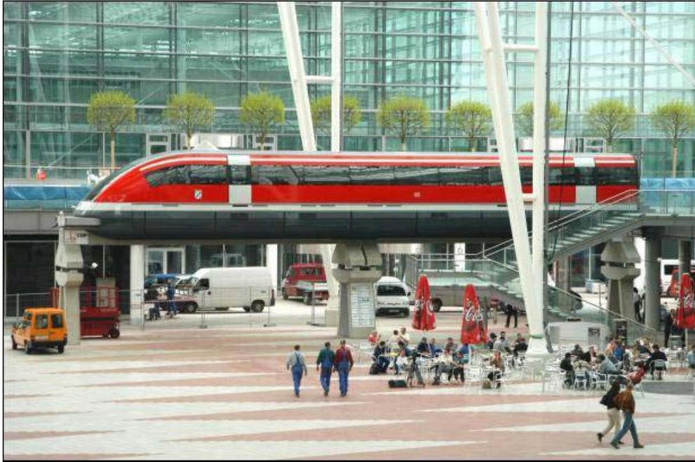
Figure 1: TR07 exhibit on a Type II hybrid guideway in the Munich Airport
