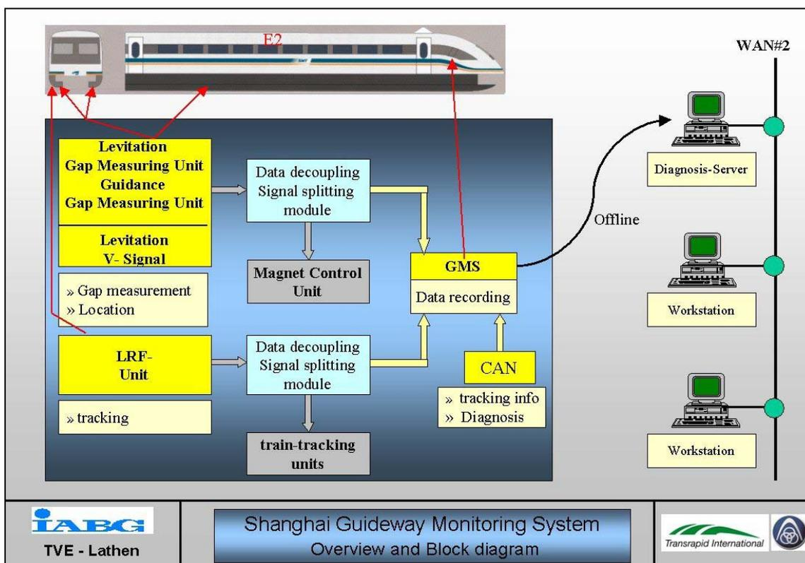
Figure 1: Block Diagram
