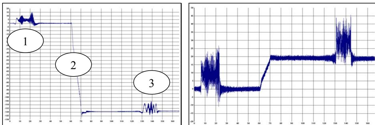
**Fig. 9 - Loads due to Bending Operation and Vehicle Passings (left: Bending Beam; right: Cantilever)**
