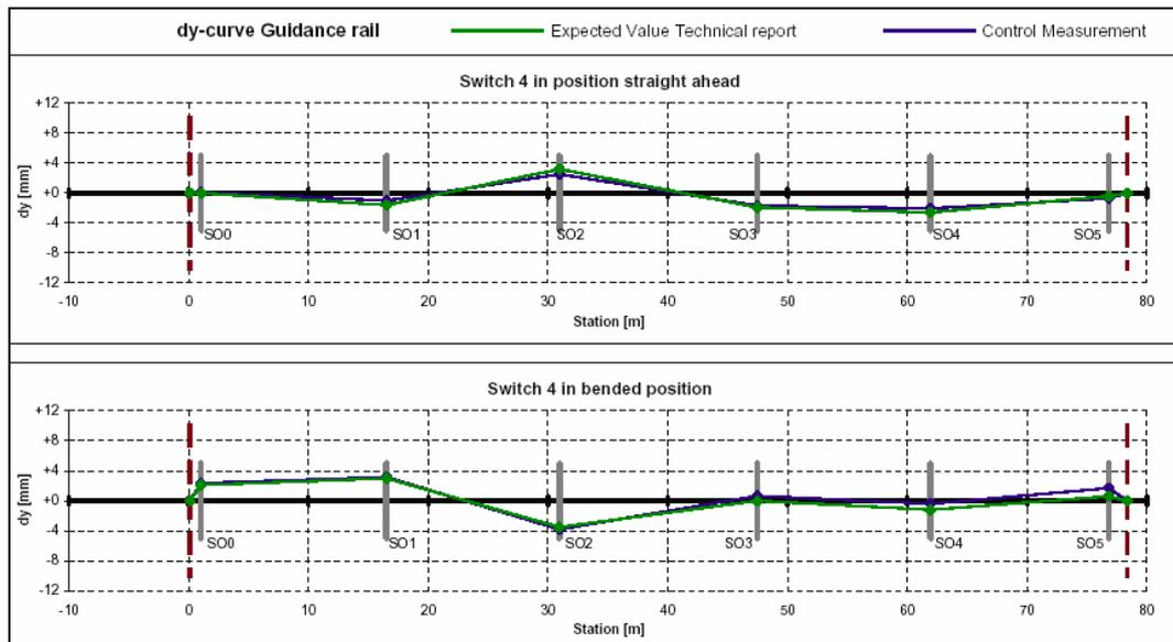
**Fig. 11 - Example of Long Wave Geometry of Switch 4 in y-Direction after the correcture of deviations**
