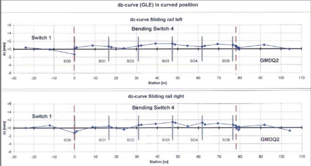
**Fig. 10 - Example of Long Wave Geometry of Switch 4 in z-Direction**
