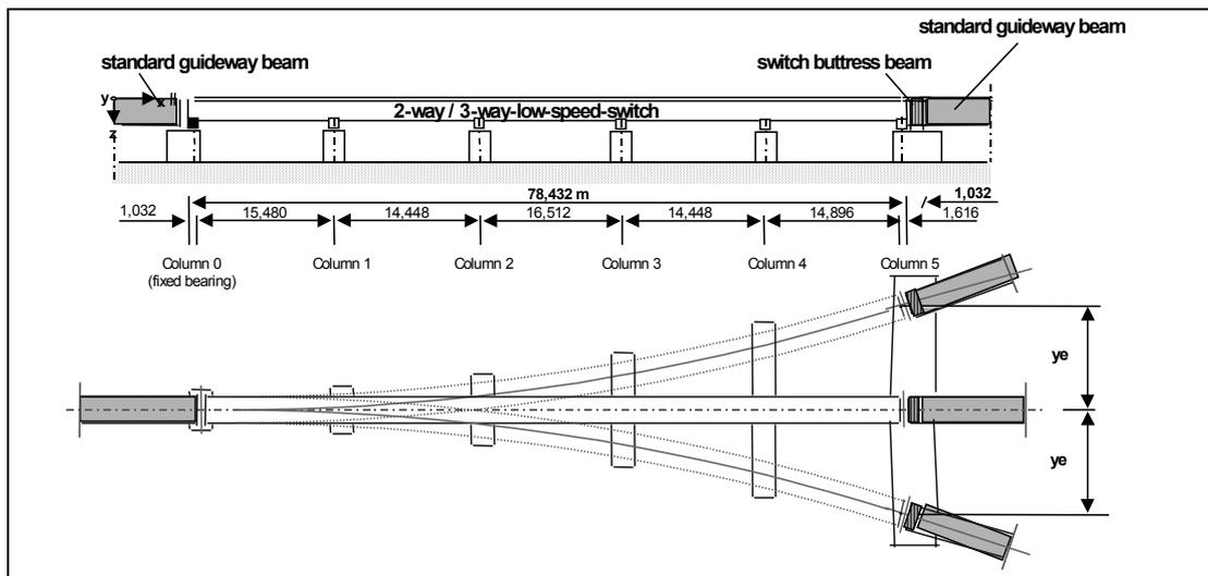
Fig. 4 - Low Speed Switch (schematic presentation)
