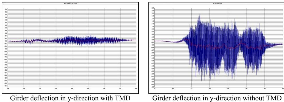
**Fig. 8 - Reduction of the Oscillation Range due to the Tuned Mass Damper**
