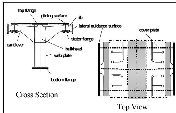
Fig. 3 - Cross Section and Top View of the 3W-LFW
