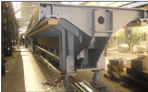
Fig. 6 - Preintegrated Girder Segment
