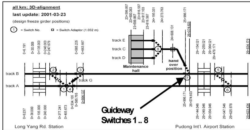
Fig. 5 - Track Scheme of the Shanghai Maglev Guideway with the Position of the Guideway Switches
