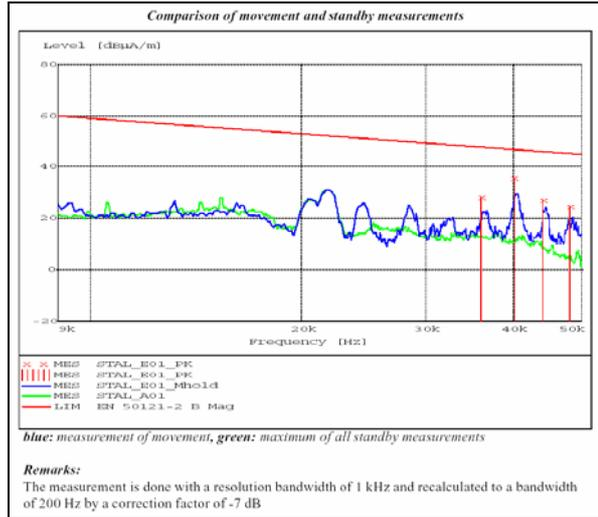
**Fig. 13 - Example of EM-Measurement Result**
