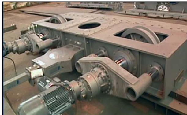
Fig. 7 - Assembled Locking and Propulsion Unit
