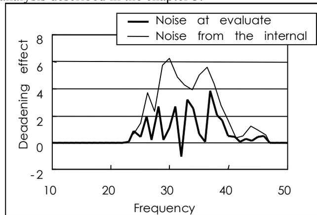
Fig. 7 Prediction of noise deadening level at the 3<sup>rd</sup> sheet by ANC system
