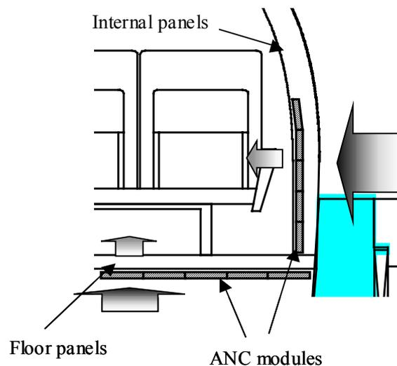
**Fig.3 Image of application of the ANC system to a vehicle**
