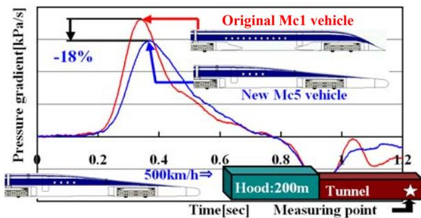
Fig.7 Comparison of pressure gradients
