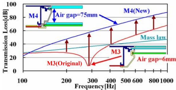
Fig.10 Calculated transmission loss of windows
