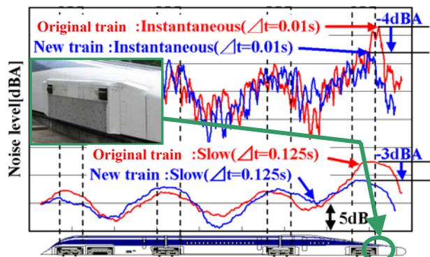
Fig.9 Comparison of outer noise
