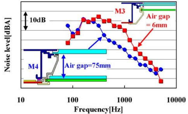
Fig.11 Comparison of noise in the cabin
