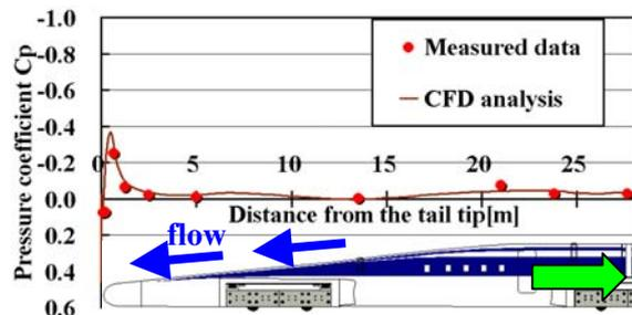
Fig.4 Surface pressure of the leading car
