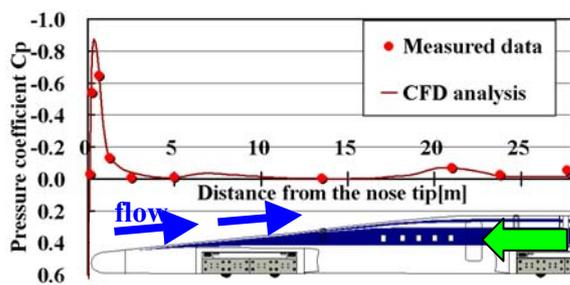
Fig.3 Surface pressure of the leading
