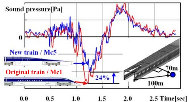
Fig.8 Comparison of low frequency noise
