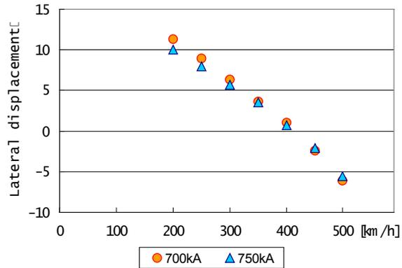
Fig2. Lateral displacement vs. vehicle speed, on a curved guideway section
