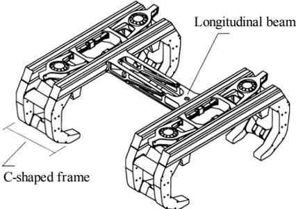
Fig.1 Bogie structure of TR08 vehicle
