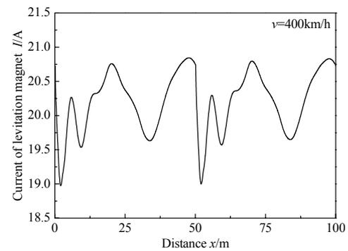
Fig.11 Current on most frontal windings
