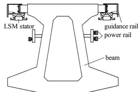
Fig.5 Cross section of maglev guideway
