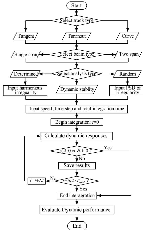
Fig.7 Flow chart of special simulation program
