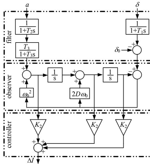
Fig.6 Block diagram of control system
