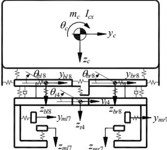
Fig.2 End view of TR08 vehicle model
