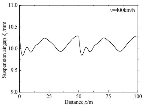
Fig.10 Levitation airgap on most frontal sensor
