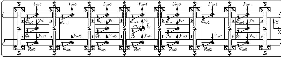
Fig.4 Plan view of TR08 vehicle model
