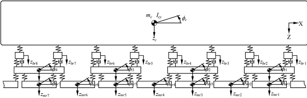
Fig.3 Elevation view of TR08 vehicle model
