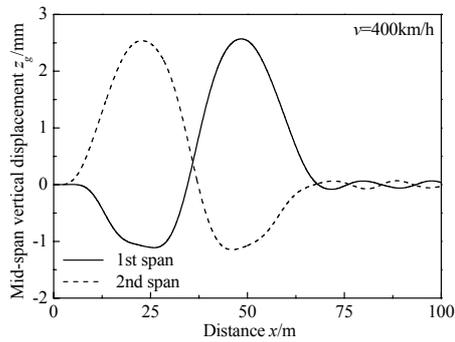
Fig.8 Midspan vertical displacement of guideway
