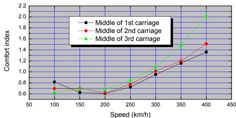
Figure 5: Evaluation results of PV2 (5-section train) on track A
