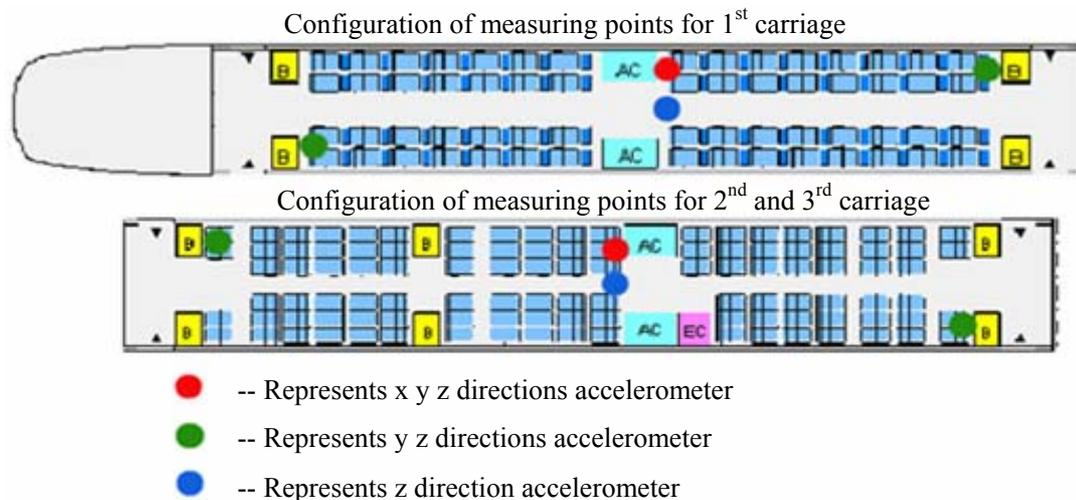
Figure 3: Configuration of measurement
