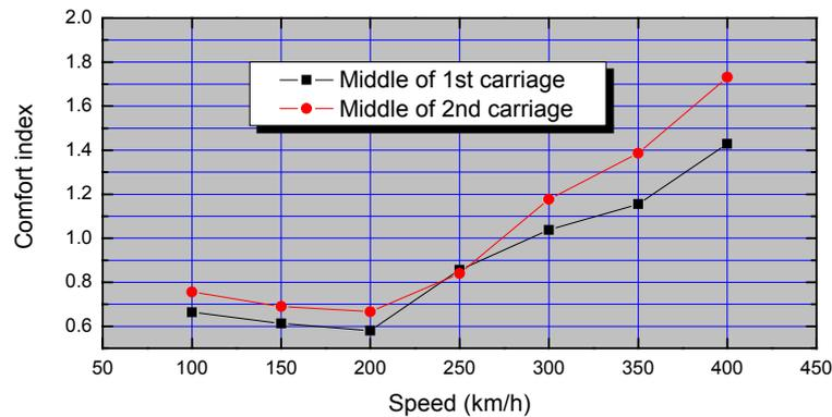
Figure 4: Evaluation results of PV1 (3-section train) on Track A
