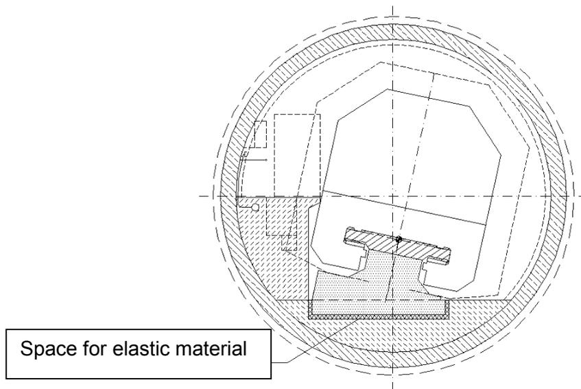
**Fig.2: Mass-and-spring system in the tunnel**
