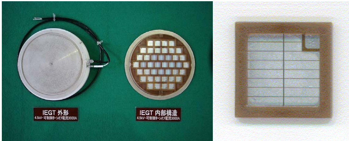
Fig.4 External form, inner structure and chip of 4.5kV-3kA IEGT
