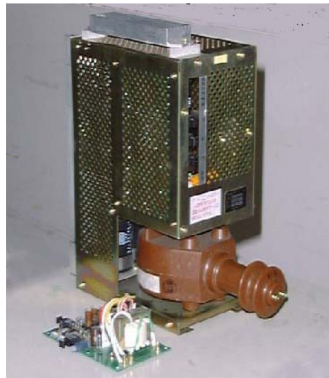
Fig.5 Gate driver unit for IEGT(left 110x165x50mm, Pin=0.13W) and GTO(right 140x219x450mm, Pin=200 to 300W at 500Hz)
