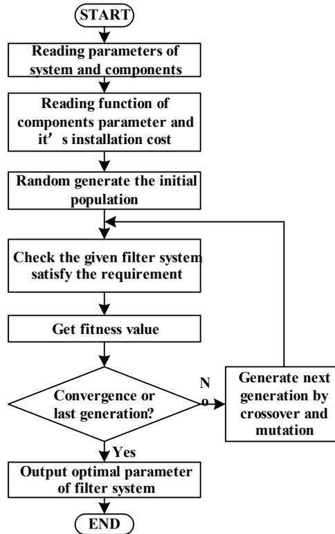
**Fig.3 Flowchart of the optimal parameters of filter system using GA**
