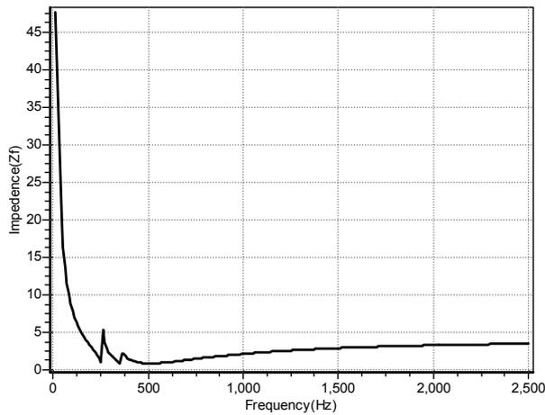
**Fig.4 Filter impedance frequency curve**
