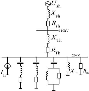
Fig.1 The schematic diagram of the filter
