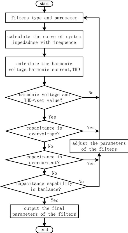
Fig.2 The flow chart of the filter system design
