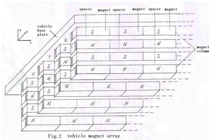
Each magnet array consists of  $n$  ( $n=1, 2, 3\dots$ ) magnet columns. Each magnet column consists of  $m$  ( $m=1, 2, 3\dots$ ) magnet strips and  $(m-1)$  spacers (Fig. 3).
