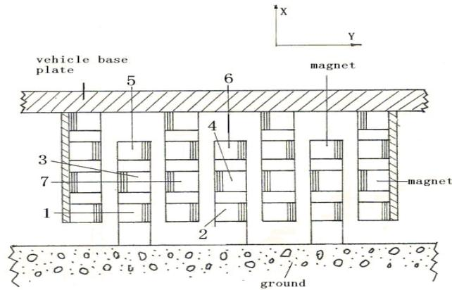
Fig. 4 The Cross-section of MAS levitation system
