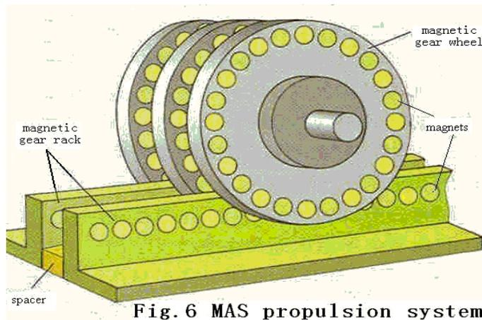
Fig.6 MAS propulsion system
