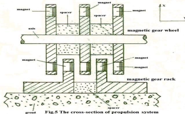
Fig.5 The cross-section of propulsion system
