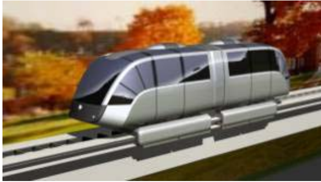
Figure 1. General Atomics Urban Maglev vehicle uses permanent magnets arranged in a Halbach array configuration for levitation and propulsion.
