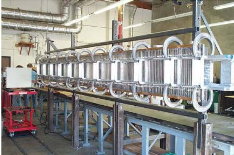
Figure 7. Semi-automated soldering process enables consistent joint resistance
