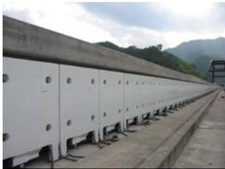
Fig. 7 Integrated type coils
