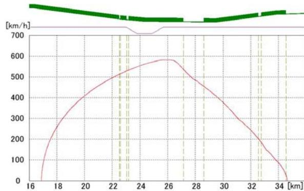
Fig. 3 Running profile of 581 km/h
