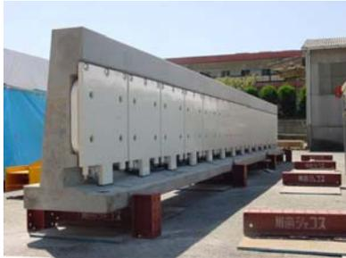
Fig. 5 Free-standing RC sidewall
