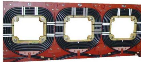
Fig. 8 Cable type coils
