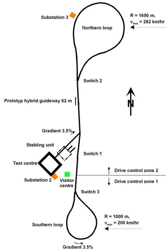
Figure 3 shows the route of the TVE guideway.
