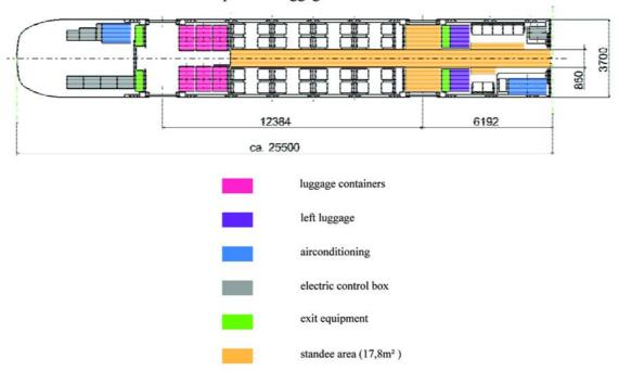
By providing room for more passengers on each vehicle (from 222 up to 412) esp. for short distance rides it is possible to reduce the number of sections or even vehicles if the fleet is big enough. By further providing larger doors the changing times for passengers can be shortened, what makes it possible to shorten the complete stop time too. For the passengers the time will be even more comfortable than now as by some actions taken such as new floor structure the inside noise level is reduced.
