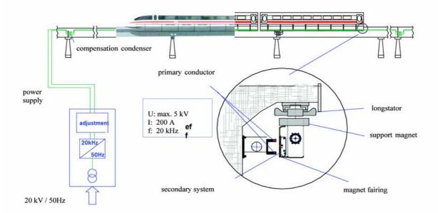
This concept will make it possible not only to provide energy transfer at all speed independent from weather conditions but as movable parts are reduced maintenance can be reduced as well. It is a system adequate development which is a step towards a new principle of onboard energy. This development has part in reducing inboard and outside noise level.
