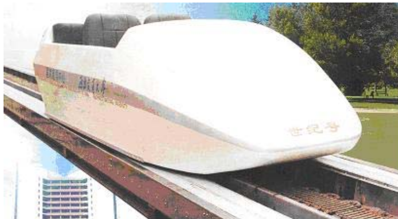
Fig. 5 HTc Superconducting Test Vehicle (developed by Southwest Jiaotong University)
