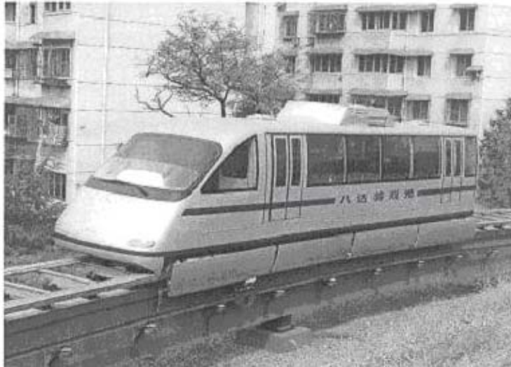
Fig. 4 HSST Type Low-Speed Vehicle CMS-03 Badaling (developed by National University of Defense Technology)
