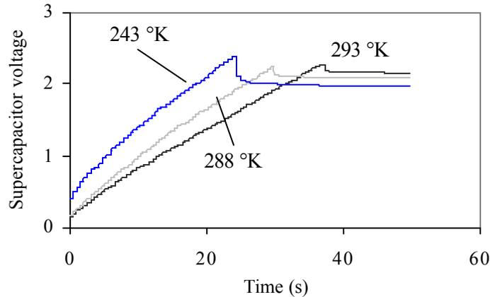
Figure 5 : Charge of 2700 F supercapacitor at constant current
