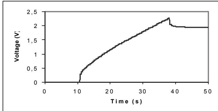
Figure 2 : Charge of 2700 F supercapacitor  $I_{ch} = 135$  A.
