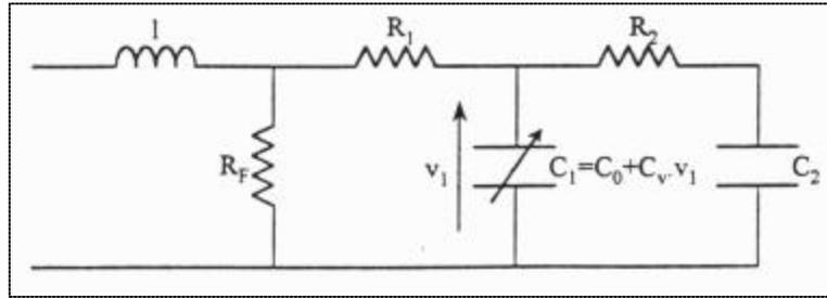
Figure 1 : Supercapacitor equivalent circuit
