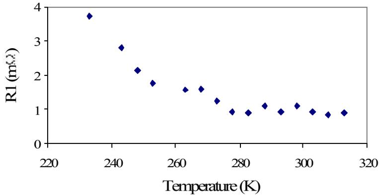
Figure 3 : Evolution of 2700 F serial resistance with temperature
