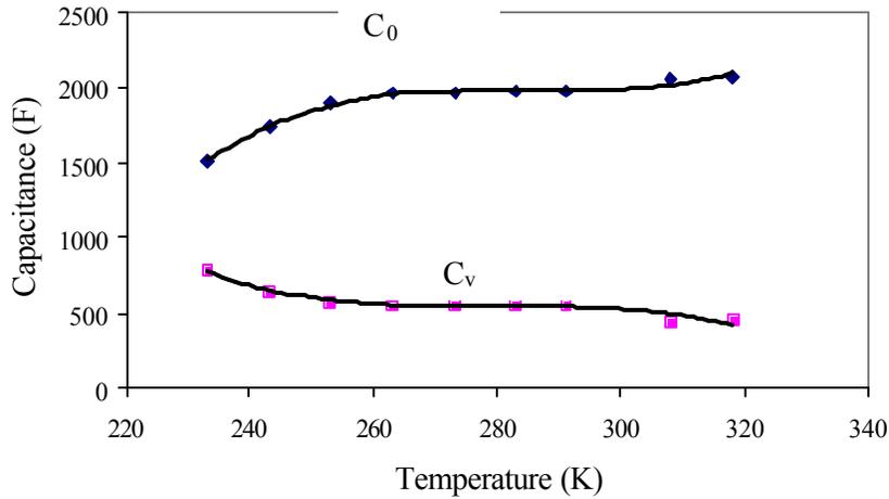
Figure 6 : Variation of  $C_0$  and  $C_v$  with temperature
