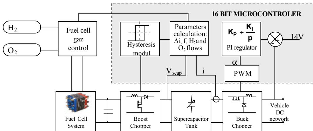
Fig. 7: General scheme of the regulation.
