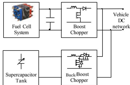
Fig. 5: General scheme of the supply (parallel structure).
