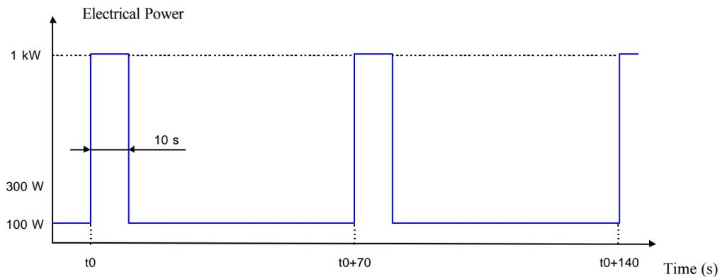
Fig. 3: Power consumption of the electric air heater.
