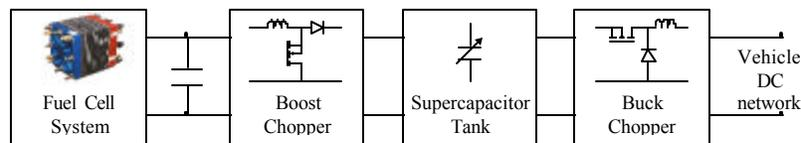
Fig. 4: General scheme of the supply (serial structure).
