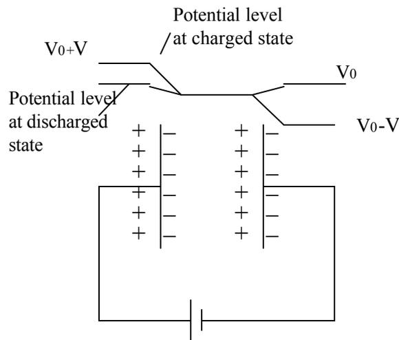
Fig. 2: Principle of a single cell supercapacitor operation
